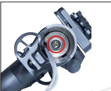
Locate the Phillips screw inside the buffer tube.
