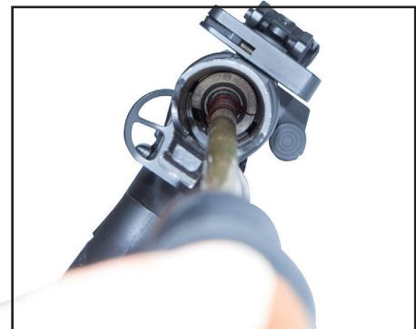
Use a long Phillips screwdriver and unscrew the screw inside the buffer tube
